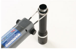
Step 4 Once the correct size has been created, connect to your Heat Inductor.
