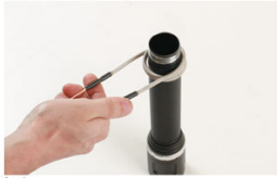
Step 3 Create a larger coil to fit over object (use 2-4 coils for best results).
